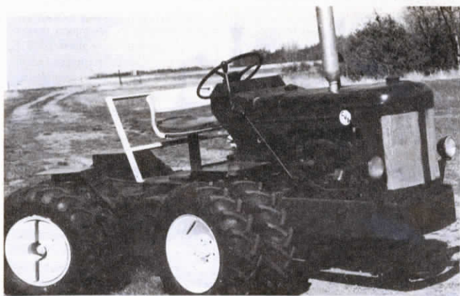
This 6-ft. long, 4-WD tractor is powered by a 20 hp Continental 4-cylinder gas engine taken from a 1944 International combine.
