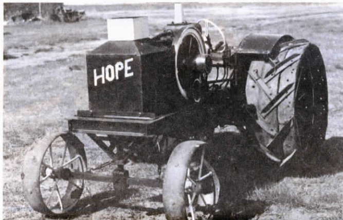
Miniature steel-wheeled Rumely rides and drives almost like the real thing and is powered by a "hit and miss" 1 1/2 hp Deere stationary gas engine.
