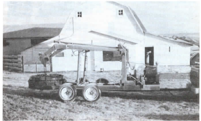
Terrance Rohr used an old Farmhand front-end loader to build his tire turner.
