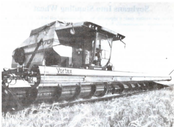
New reel takes just an hour to install and uses existing reel controls. Small-veined blower fan runs across whole width of header.
