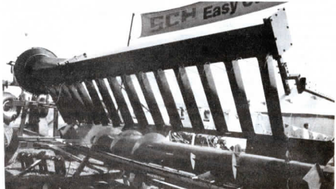
Key to success of new air system is a first-of-its-kind turbine blower that develops more than twice as much air flow with a minimum of horsepower.
