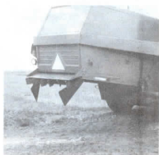
Add-on straw attachment makes a tight windrow that’ll stand up to 45 mph winds.
