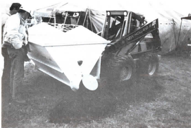
The 40 cu. ft. hopper weighs 420 lbs. and holds up to 1,200 lbs. of feed.
