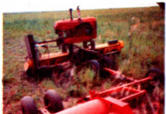
Left hand mower has front end of Massey 44 tractor mounted on top of it.
