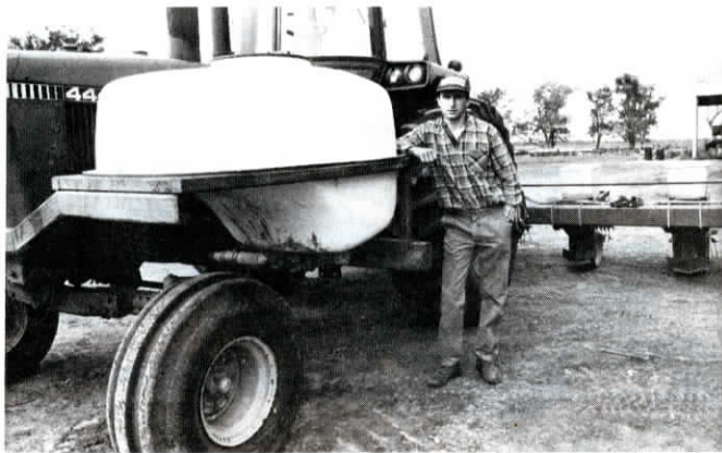
Water is pumped from two 250-gal. saddle tanks to a manifold on top of planter that splits the flow eight ways, one tube going to each row unit.
