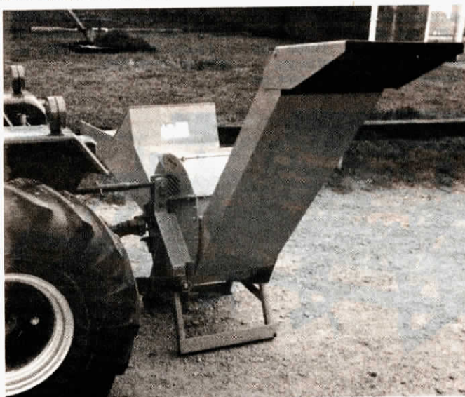
Cutterhead in home-made chipper was salvaged from a junked one-row No. 10 IH "direct throw" chopper built in late 1950's.
