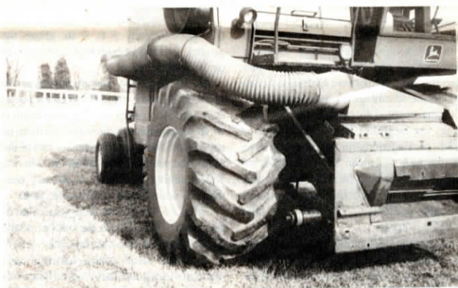
Diverter mounts over feederhouse door. A 12-in. fan sucks dust off return chain.
