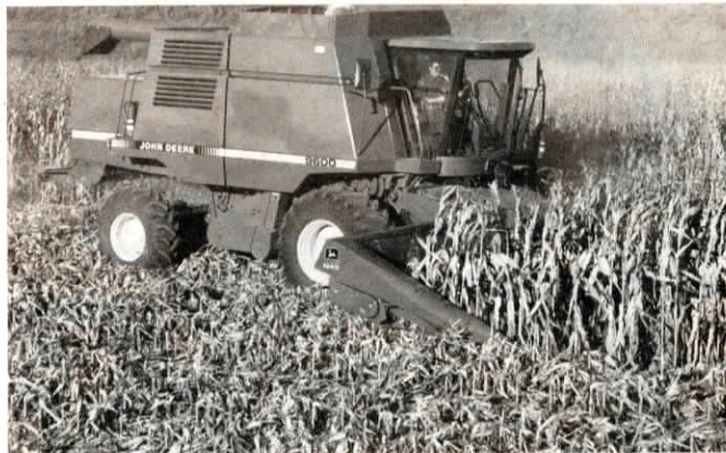
Deere lengthened the feederhouse on its new 9000 series combine to move the header forward, making it unnecessary for the operator to lean forward to see cutterbar or header height.
