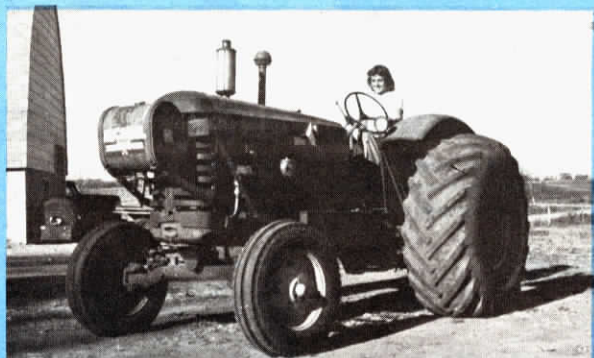
Alan Zeithamer's 12-year-old sister Ann rides the family's Massey-Harris diesel, which has run on a mixture of 50% alcohol, 50% diesel fuel for several months. Note extra fuel tank up front for alcohol, needed with the half and half mixture. Building to left is alcohol plant.
