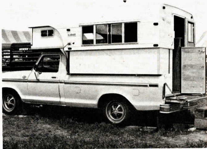
Hand-operated cylinder raises camper to its full height.
