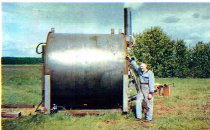
Big round bales are loaded into the 5-ft., 8 in. dia. burner by forklift. Rate of burn is controlled by electric blowers that feed in combustion air as needed.
