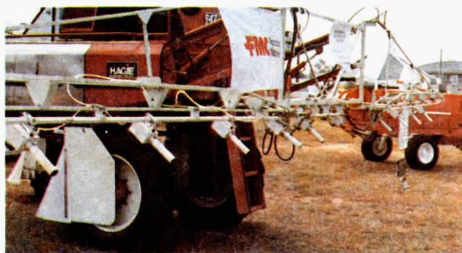
Individual row units zap spray droplets with negative electrical charge, which are then attracted like magnet to positively charged plants.
