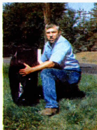
Crombie shows how collector folds to compact, 30 lb. bundle for storage, transport.
