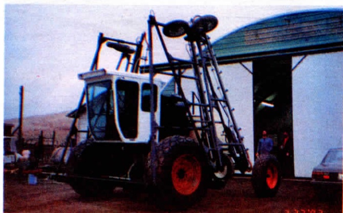
Sprayer's 92-ft., 6-section boom hydraulically folds to 18-ft. width from cab.
