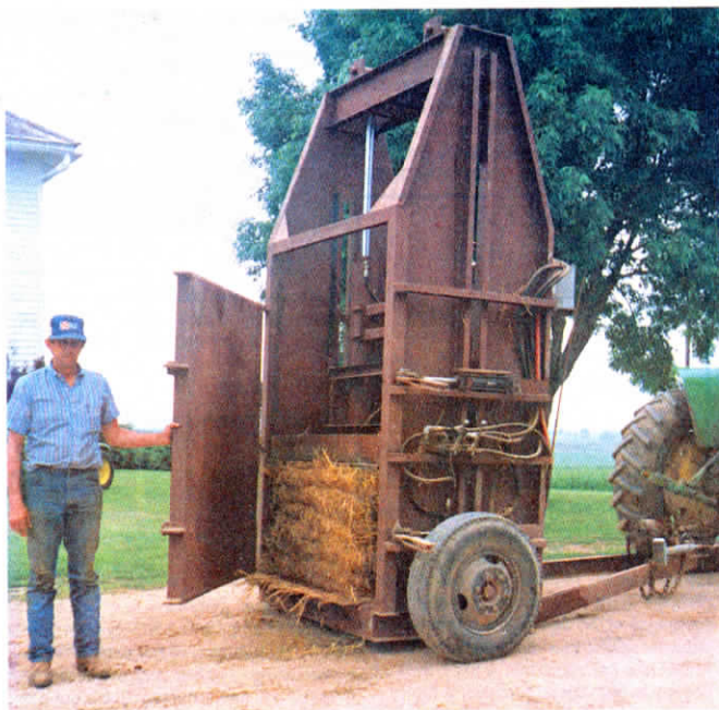
Two-wheeled compactor is powered by a pto-driven hydraulic pump. A pair of 26-in. cylinders apply 60 tons of compaction pressure.
