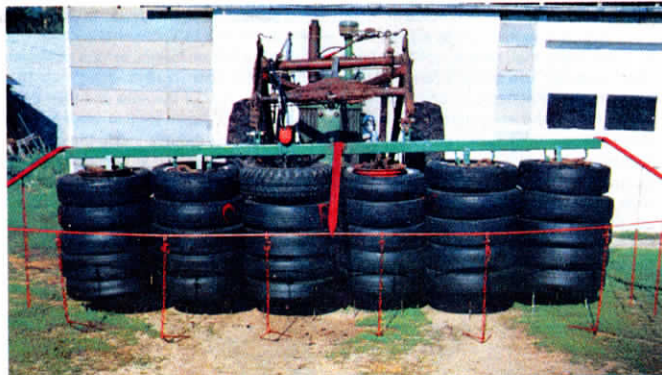
A drive chain wraps around tread of top tire in third stack from the left. It rotates that stack, which in turn drives all the other stacks.
