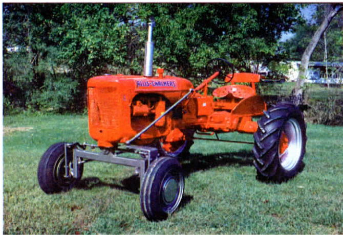
Photo shows an Allis Chalmers "C" that's been fitted with Powell's wide front axle.
