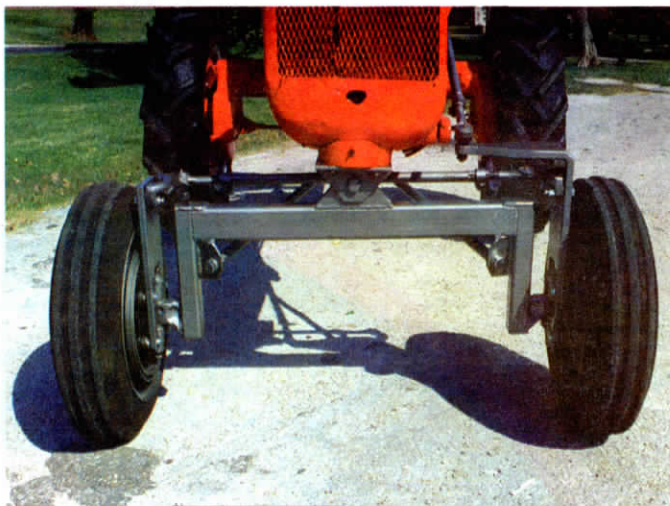
Axles are made of heavy-wall steel tubing with heavy-duty tie rods.
