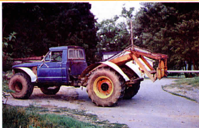
Cate built his "Jeepor" out of a Jeep pickup fitted with tractor and combine tires. A dual-purpose hydraulic lift system mounts on back.
