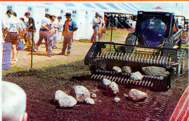
Bucket is equipped with a rotating reel that helps scoop rocks off the ground. Dirt drops out through tines as rocks slide into back of bucket.
