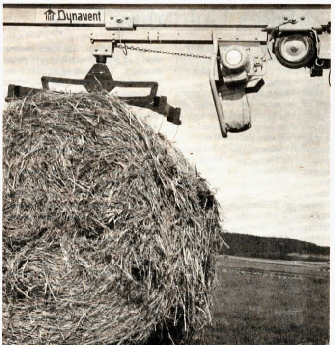
A giant claw picks up bale and an electric motor "self-propels" bale along track.
