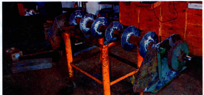
Steel discs were welded to combine cylinder shaft. Large sprocket at end of shaft is chain-driven off pto.
