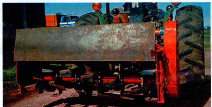
Conventional tiller blades bolt to discs on shaft. One problem with the design was that the chain guard keeps tines from working deeper than 3 in. If he did it again, Hango says he'd use a smaller drive sprocket.
