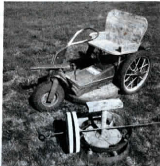
Carlile bolted an angle iron "tongue" to mower's front steering fork and runs a large rubber band from the tongue up to the steering yoke to keep the front wheel from moving back and forth.
