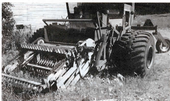
Spielman mounted a tractor-pulled rock picker on front of his 1982 Deere 2320 self-propelled swather and equipped the swather with big flotation tires.
