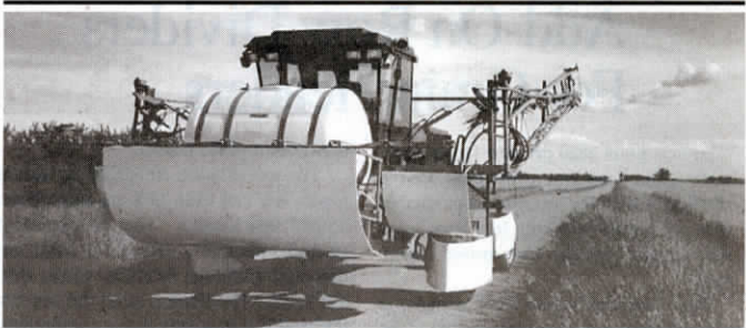
To convert a swather, sprayer unit is equipped with 500-gal. tank, sprayer booms, frame, and mounting brackets. Note protective shielding on front.
