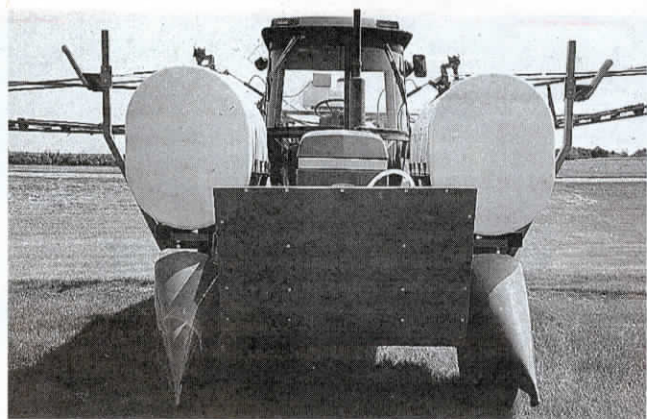
Tractor kit consists of two 240-gal. saddle tanks, narrow 9.5 tires, poly shielding underneath and in front of tractor, and poly dividers ahead of front and rear wheels.
