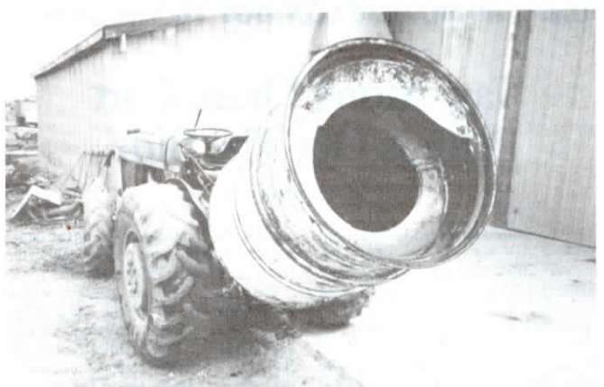
Inside the rims, he installed 4-in. spiral flighting made out of 3/16-in. sheet metal.
