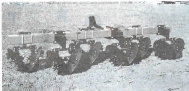
The Row Stalker consists of a set of round steel blades in a V-shaped configuration like disc openers.
