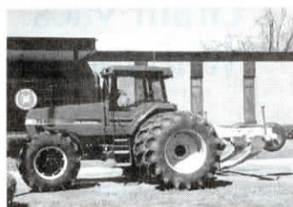
Tupper says in tests the subsoiler can always be pulled one gear faster - sometimes two - than the Paratill.
