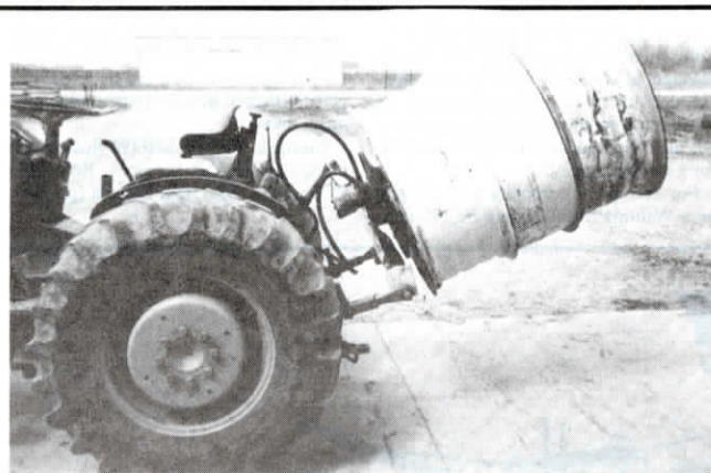
Lepp welded two 38-in. tractor wheel rims together with a spacer between, then welded the combined rims onto the backing plate of a truck spindle.
