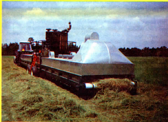
When hay exits the back of machine, it's dry enough to bale yet it's not brittle like sun-dried hay so there's almost no leaf loss, says inventor Harold Herron.
