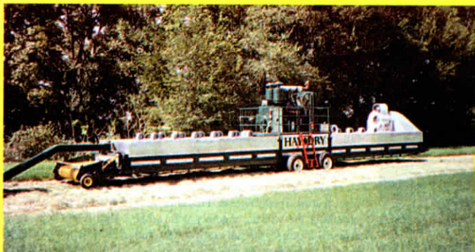
A 7-ft. wide up-front pickup reel lifts wet hay onto conveyor belts that run the length of the 50-ft. long first-of-its-kind microwave hay dryer.
