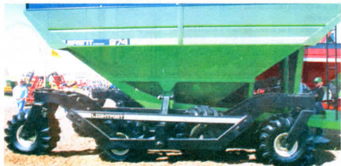
Eight-wheel transport system mounts under Unverferth's new 1,000-bu. wagon.
