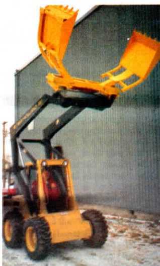
Bale grabber can be equipped with bolt-on pans that convert it into mini clam bucket for hauling rocks, brush, etc.
