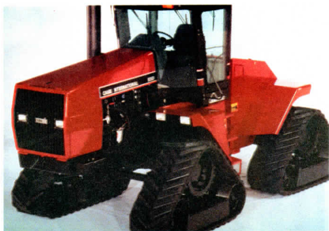
Prototype "Quadtrac" has four sets of rubber tracks that mount in place of wheels.
