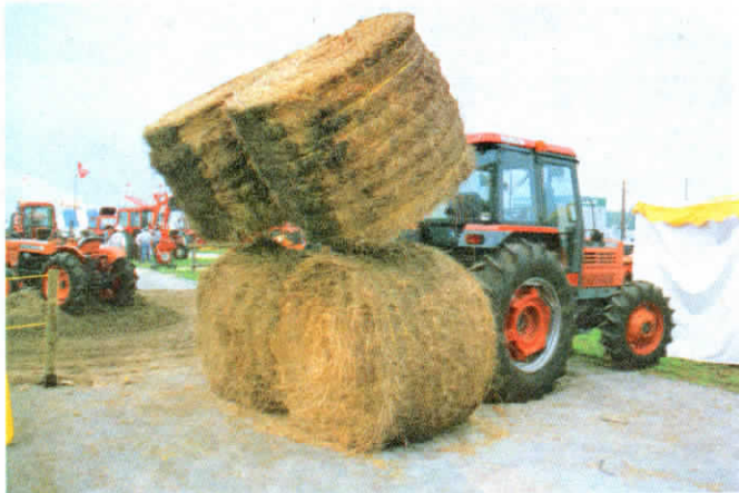
Two steel forks mount one above the other on new 4-bale hauler.
