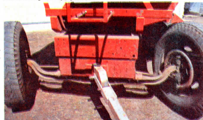
Kamen removes the springs from the front axle to reduce sway.
