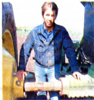
Kelly Blair widened his tractor axles so they'd match the width of his combine wheels. He uses all 8-row equipment and always runs in the same two rows.
