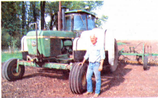
Roger Hade widened the front axle on his Deere 4640 to 120 in. and turned the rear wheels around so they'd also be spaced 120 in. apart.
