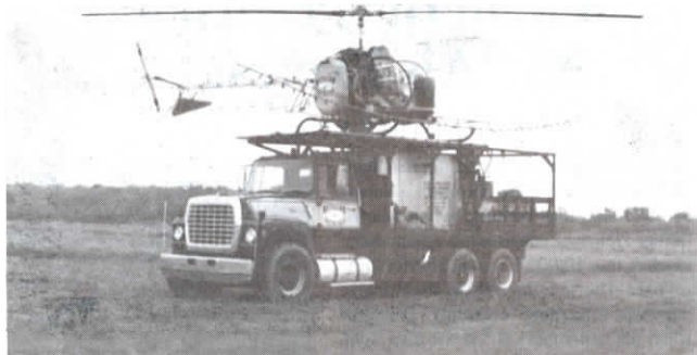
Squires lands his helicopter crosswise on truck-mounted pad to load up chemicals.
