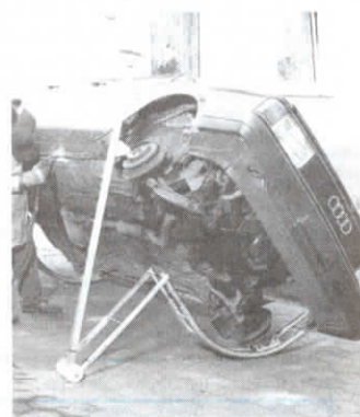
Two rocker panels go on one side of car. Lifting device bolts to front hub on opposite side.
