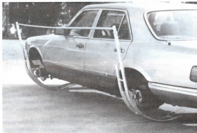
Side view shows how rocker panels are held in place by two lug bolts on each wheel hub.
