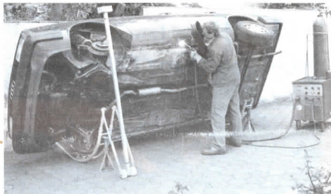
“Tilter” tilts car up to 90 degrees. To set it up, you remove three wheels.
