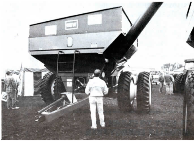
Adding a second set of tires reduces soil compaction by 20 to 50%, says company.
