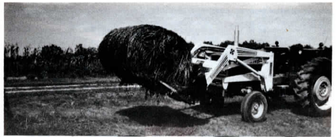
Fork’s teeth, 36 in. long and spaced 10 to 12 in. apart, are secured by bolts.
