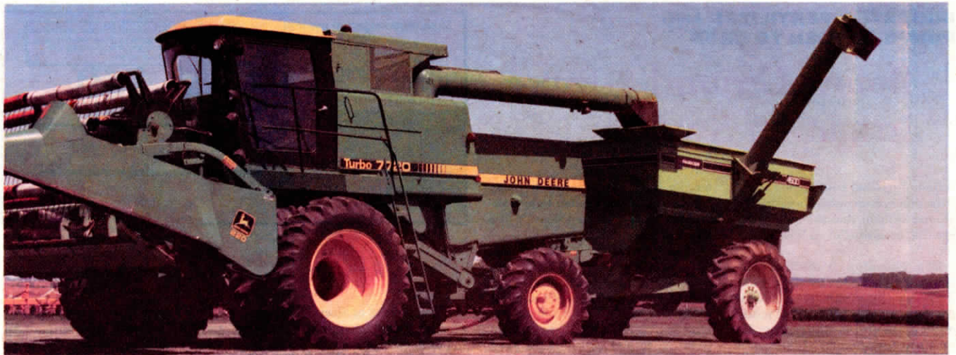
When combine grain tank fills, it's unloaded "on the go" into the trailing grain cart.
