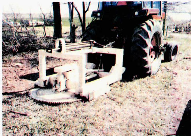
Tree saw blade (48 in. in dia.) moves into the tree automatically as it cuts deeper.
