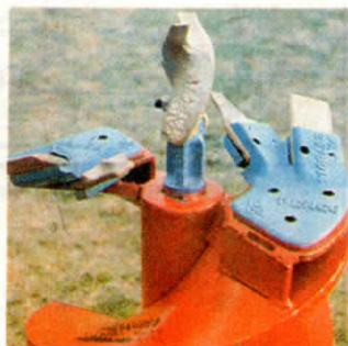
Tungsten carbide teeth can be installed to dig through frozen ground, if required.
