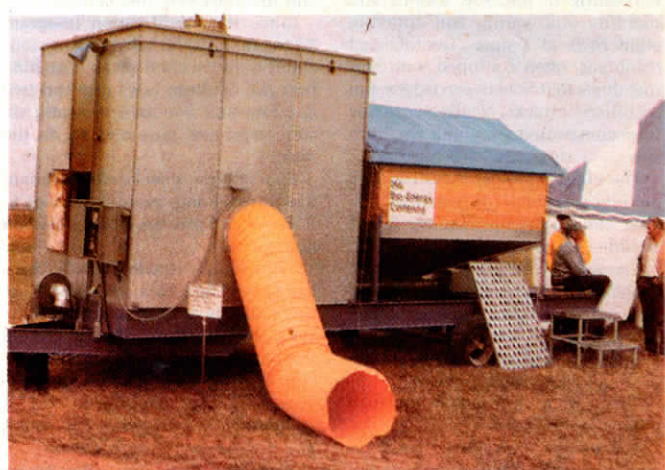
Temperatures inside stainless steel burning chamber reach up to 2,500° so that less than 2% of residue is left to be cleaned out.
