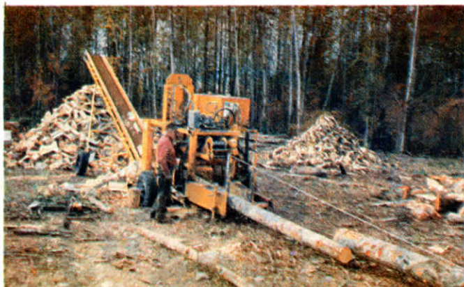
Hydraulic shear blade cuts the log and then also pushes it onto splitter head, simultaneously pulling the log up for the next cut.
