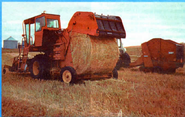
Joe Laczko put together this self-propelled round baler by stripping down a Massey 510 combine and mounting a baler on back. He amazed friends and neighbors by building the round baler himself entirely from scratch.
