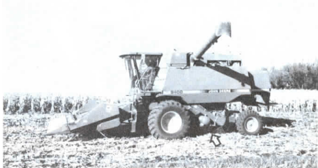
Little Duster stores oil in 15-gal. tank mounted on side of combine (see arrow).
