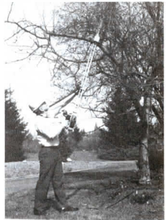
New chain saw trimmer lets you trim tree branches up to 10 ft. high while standing on the ground.
