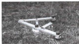
Spring-loaded pulleys connect wires on the sleds with electrified side fence wires.
