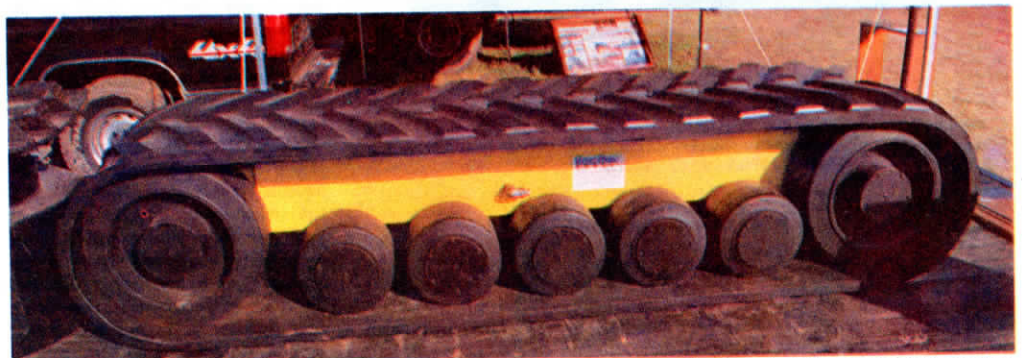
Gilbert & Riplo's non-powered undercarriage can be fitted to manure spreaders, spray tanks, grain tanks, and other equipment.
