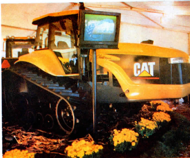
This new Challenger 45 tractor is fitted with 18-in. wide belts.
