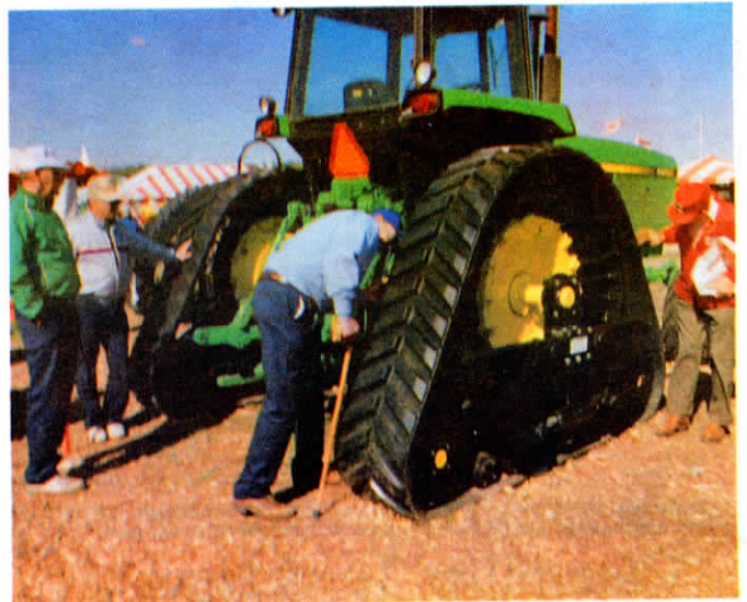
Kelderman's direct-drive tracks have a built-in hydraulic suspension system.
