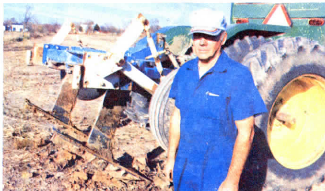
Ross says he's literally changing his soil profile with this tool built out of a DMI ripper with a pair of 4-ft. long shanks fitted with "spader" blades.
