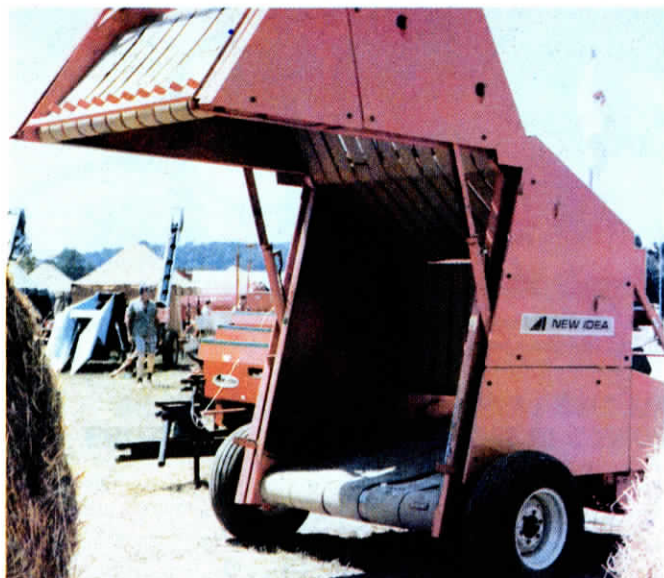
New Idea baler makes 6 ft. dia. hay bales measuring about 5 ft. wide and weighing about 1,800 lbs.
