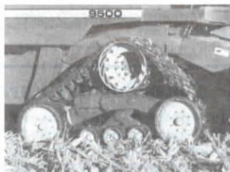
Four pivot points allow rubber tracks to conform more closely to soil surface for better traction and ride comfort.
