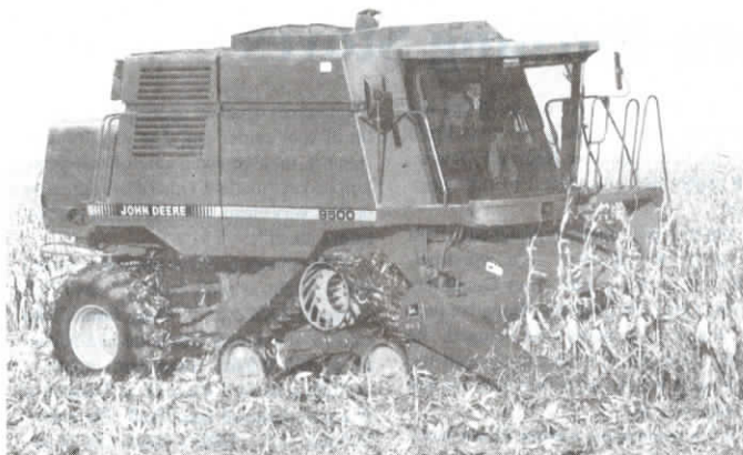
Deere is offering new rubber tracks designed for its 9500, 9600, and CTS combines.
