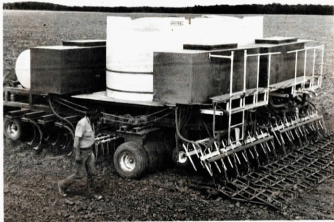
Giant drill applies 250 gal. of "pop-up" water per acre injecting it into the row right along with the seed.
