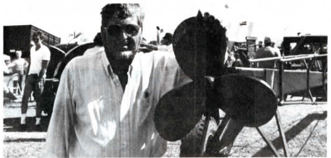
The 22-in. prop's blades have a 3-in. pitch, says Denny Ortel, owner.
