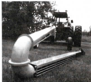
Self-contained auger trails behind a tractor or pickup for road travel.
