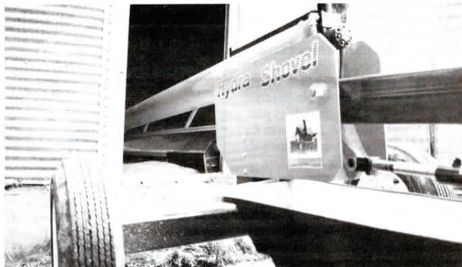
Hydra Shovel cleans bins from 14 to 22 ft. in dia. and unloads into any transfer auger.
