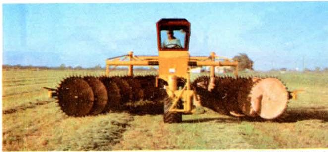
Rake is powered by 52-hp. Deutz engine. Covers a 16-ft. swath at speeds up to 15 mph.
