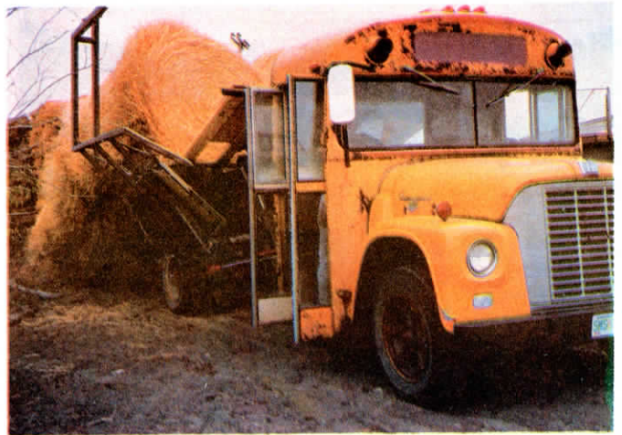
Side-mounted bale loading arm is made out of 2-in. tubing. Bus holds 6 bales in two rows and unloads them off the back by hydraulically tipping deck.
