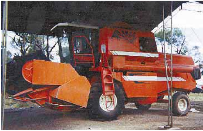
Combine's 150 hp diesel engine uses only 3 1/2 gal. of fuel per hour.
