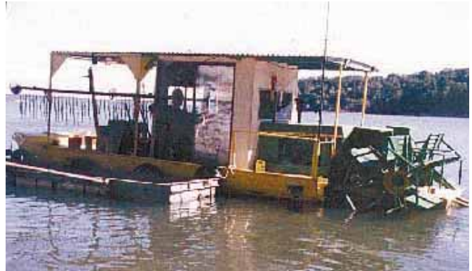
Swather's wheels are fitted with 4-ft. wide paddle wheels that Deering made from the batts on the original swather reel.
