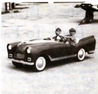
Geared-down two-seater “toy” car is powered by 5 hp single cycle engine and has 3-speed transmission from 1941 Packard car.
