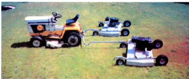
Three-bladed 57-in. wide decks are powered by 12 1/2 hp electric-start engines.
