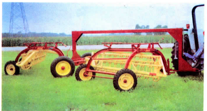
Rear rake is towed by bridge hitch connected to combine steering axle fitted with power steering. Rake moves from side to side by turning the wheels hydraulically.
