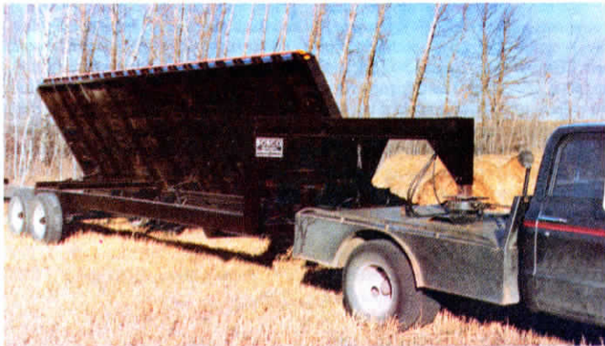
Three hydraulic cylinders tilt deck up to left side for quick unloading of bales.
