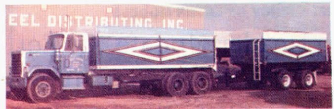
Converted semi tractor, with pup trailer, provides “capacity of a conventional semi at a lot less cost and is much more maneuverable.”
