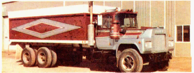
Semi tractor is stripped of its fifth wheel and the frame lengthened to the desired wheelbase.
