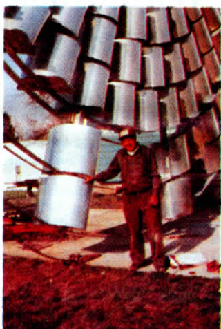
Individual air foils in Gerhardt's windmill are 2 ft. wide and 6 ft. in circumference.
