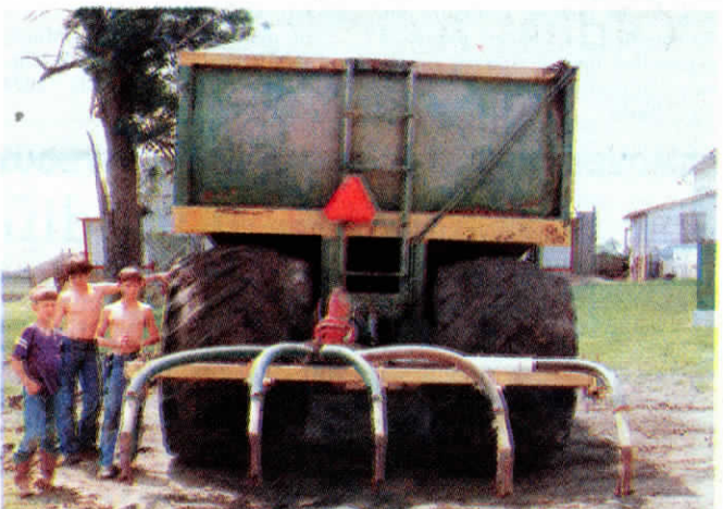
Manure is pumped through 3 in. hose to a manifold which distributes it to 5 soil injection knives.
