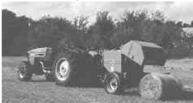
Mini baler makes 3-ft. wide, 2-ft. dia. bales. A 3-pt. hitch wrapper is also available.
