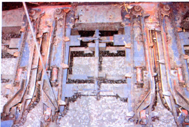
Adjusting mechanism mounts directly under each snout (snout removed in photo) between every two rows. Rotating shaft has two linkage arms attached to either end of it that attach to the stripper plates on each side. Hydraulically-controlled sliding tube under head turns rotating shaft, opening or closing stripper plates.
