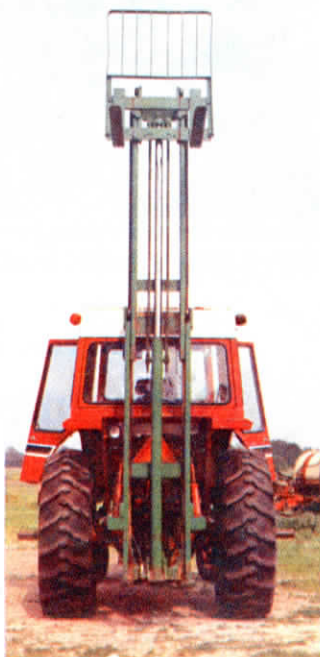
Zelhart adapts 2 and 3-stage forklifts, with up to 20 ft. of lift, to mount on 3-pt.
