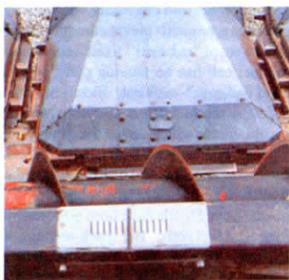
Photo shows indicator gauge that's clearly visible from cab. Scale is marked in 1/16-in. increments.
