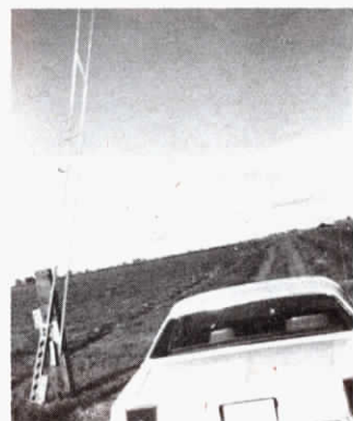
Revving up engine on a "hornless" tractor will activate sensor to automatically open or close the gate.
