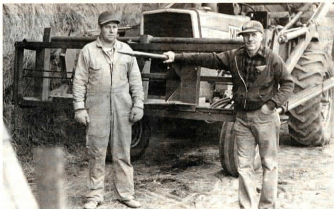
A hydraulic-driven chain shifts the bale spear back and forth to easily stack bales in corners and up against the side of the pole shed without moving the tractor.
