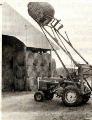
Modified Farmhand hay stacker, equipped with home-built "side shift" loader, stacks bales 5-high.
