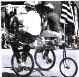
Hull's "Hullarious Trike" is a big hit in parades. Pedals direct-drive wheels.
