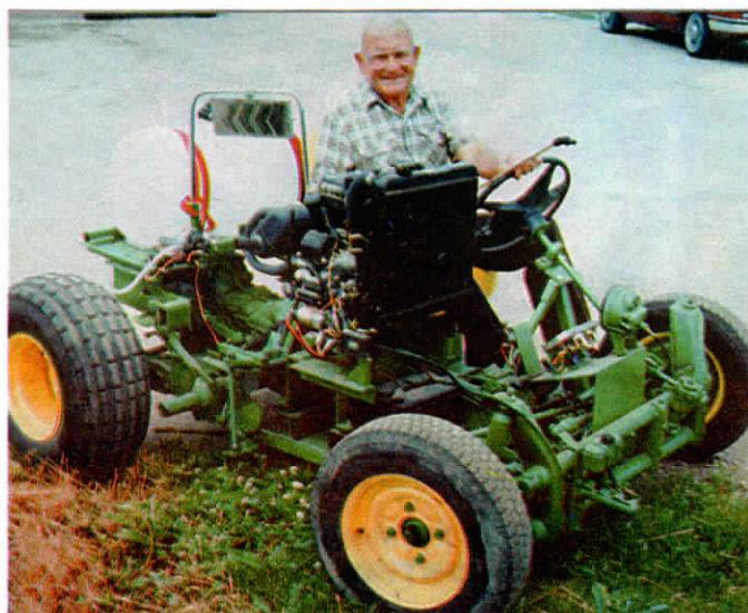
Uhnken used parts from a pair of junked Volkswagen cars to build "wide-track" ATV. He uses it for spot spraying in soybeans and to seed waterways and terraces.
