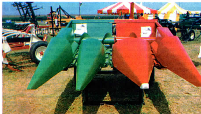
Plastic shields are lighter in weight and less expensive than metal gathering shields.
