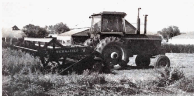
For about one-fourth the cost of a self-propelled swather, Arlen Foster adapted a Versatile header to his turned-around tractor.
